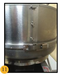
Attach the retaining ring to the outside of the mixing drum and secure by latching the retaining ring clasp to ensure a tight fit.
