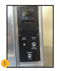
After the final steam clean, turn the machine OFF, unplug the unit and allow it to cool before cleaning. Make sure to clean all pans/accessories in order to sanitize them before each use.
