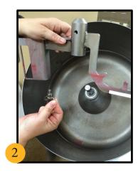
Remove paddle via the small wing nut lock stud. The paddle can be washed in a sink or dishwasher; also the small silicone scraper can be removed via the 2 small wing nuts holding the scraper retainer.
