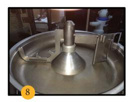
Once kettle is clean, replace clean paddle and wing nut onto the agitator shaft.
