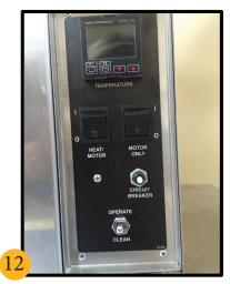
Switch the toggle to the OPERATE mode. The machine is now ready for use.
