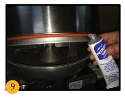
Take the drum seal and place a small amount of Petro Gel all around the drum seal and place seal on the lower level of the mixing drum. DO NOT stretch the seal out.
