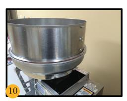
Place the mixing drum with the drum seal back on the kettle. The bolted side of the drum should be on the non-pour side.
