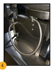
Wipe the kettle lead cord with a clean SLIGHTLY damp cloth. DO NOT get moisture into the kettle leadin cord, severe damage will result.
