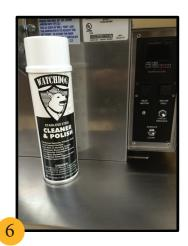
Wipe the stainless steel parts with a clean cloth and cleaner designed for stainless steel such as Gold Medal Watchdog Stainless Cleaner (Item No. 2088). DO NOT USE OVEN CLEANERS OR ABRASIVE MATERIALS.
