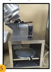
The cabinet/table the machine sits on should be wiped clean daily with a clean, slightly damp soft cloth.
