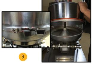
Release the draw latch to easily remove the mixing drum, then take to the sink to clean. Remove drum seal and clean if needed.
