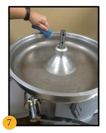
Wipe out kettle and rim once the drum is removed.
