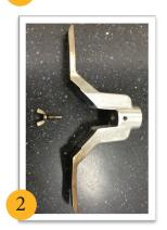
Remove paddle via the small wing nut lock stud. Remove any burrs on the shaft using a fine grit emery paper to lightly sand the surface. If burrs are not removed, damage may occur to the o-ring/oil seal during removal/installation.
