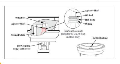
With the machine OFF, unplug the unit and allow it to cool before attempting to clean the Hub Seal Assembly.
