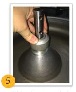
Slide the clean hub seal down the agitator shaft. Apply pressure to ease the assembly over the center hub of the kettle until it seats properly.
