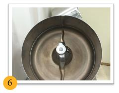
After the hub seal assembly has been properly installed, re-install the mixing paddle onto the agitator shaft. Finger tighten the wing bolt to secure the mixing paddle in place.
