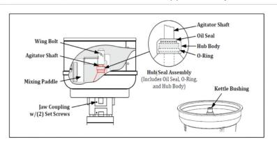
With the machine OFF, unplug the unit and allow it to cool before attempting to clean the Hub Seal Assembly.
