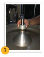
Remove the hub seal assembly and soak it in hot water to clean. Clean the area around the center hub and remove any product residue.
