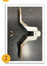
Remove paddle via the small wing nut lock stud. Remove any burrs on the shaft using a fine grit emery paper to lightly sand the surface. If burrs are not removed, damage may occur to the o-ring/oil seal during removal/installation.
