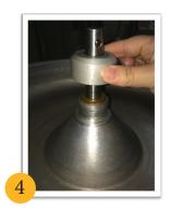
Lightly lubricate the center hub of the kettle with a small amount of vegetable oil to allow for easy re-installation of the hub seal assembly.
