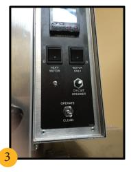
Turn Heat/Motor Switch ON and ensure toggle switch is in the CLEAN position; the preset set point temperature is 230F.
