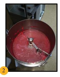
Carefully pour in enough water to fill the kettle to right below the drum seal. This should be approximately 1.75 gallons. The water should be warmnot cold to avoid damage to the kettle.
