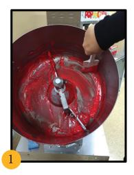
After all product has been removed, with the machine OFF, use spatula to scrape as much access dried fudge as possible from inside the kettle and around the paddle.
