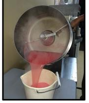
Allow unit to cool, then remove lid and carefully pour dirty water into a bucket, discard appropriately, then wipe inside of kettle with a clean cloth or paper towel to finish cleaning. For extremely dirty kettles, we recommend running a 2nd cycle.
