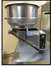
Put the lid on the kettle and let the machine run for approximately 20 minutes; the kettle will steam and wash the residue into the water, the turn the Heat/Moto Switch OFF.
