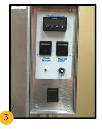
When the water starts to boil, turn the Heat/Motor switch OFF and allow the kettle to cool.
