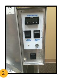
Place the lid on the kettle and turn the Heat/Motor switch ON.
