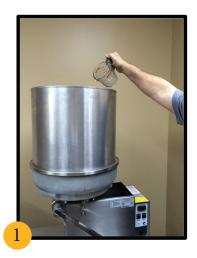
After all product has been removed, and the kettle has cooled for 15-20 minutes, carefully pour 24oz of warm water into the kettle.
