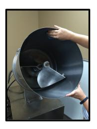
Once the water has been removed, wipe out any access sugar build-up from the kettle using a damp rag.
